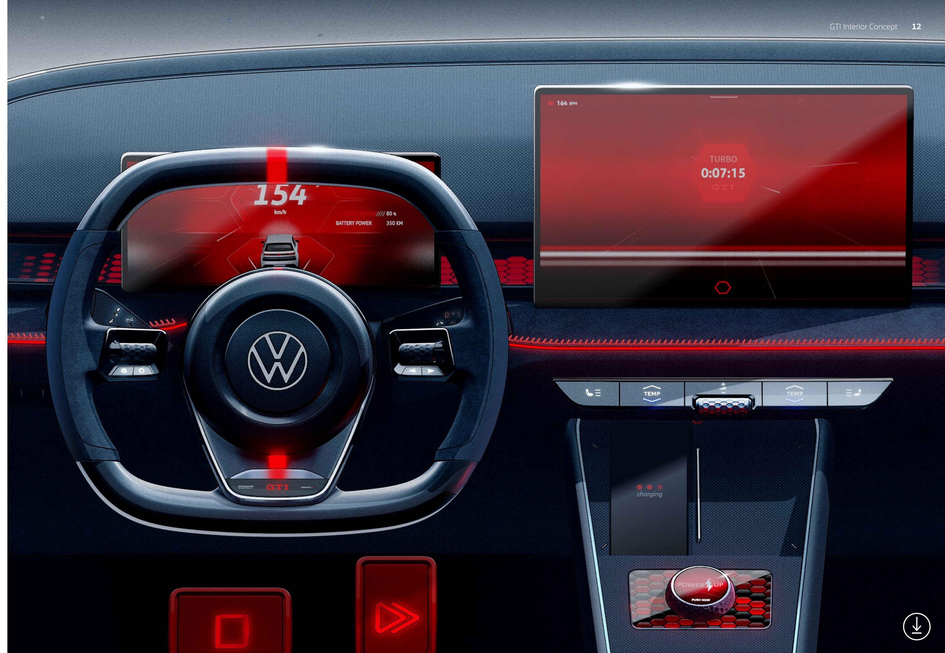
GTI steering wheel: the airbag design is a homage to the first GTI. The 12 o'clock marker and the special GTI button is illuminated in the colour GTI Red Turbo
