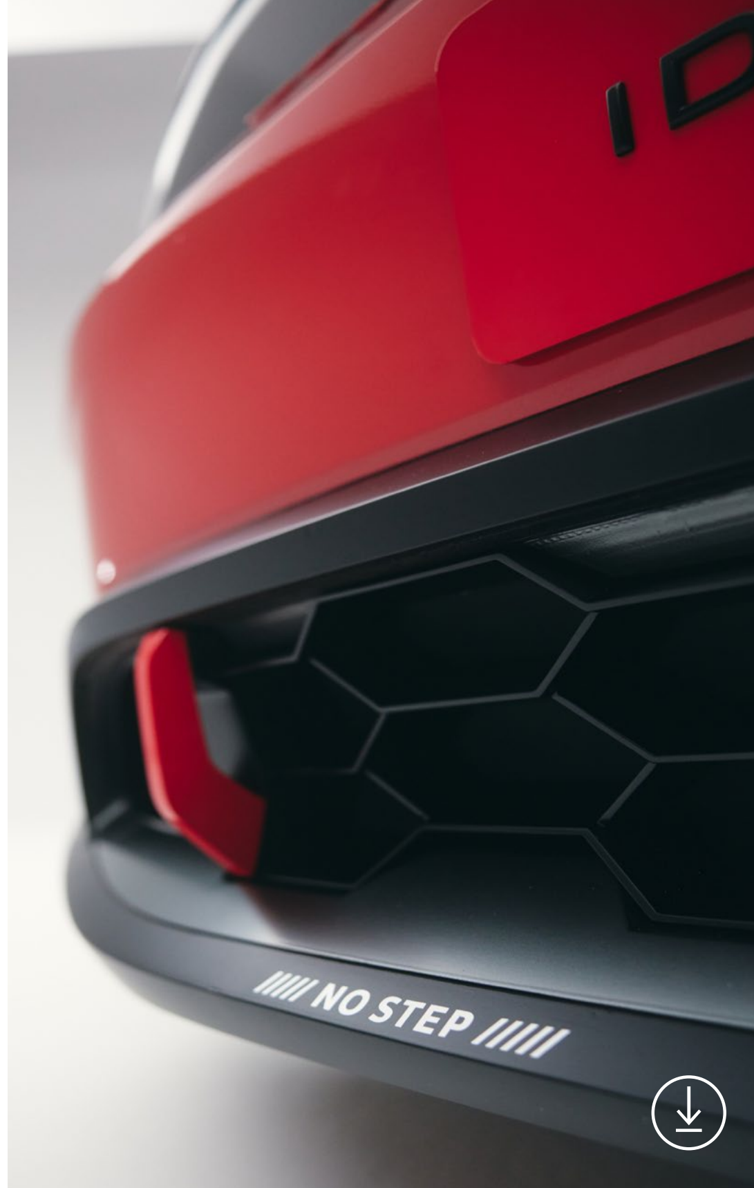
GTI spoiler: a splitter increases the downforce
